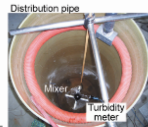
Large mixer for the suspension of sediment in water (1 m diameter)
