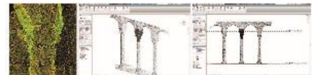
Figure 2. Characterization of a dome with repeated arches (left) in a mesh (middle) containing 100k points without any data plug-in; points are clustered to detect sort of "holes" and irregular geometry that cannot be processed in a regular way; a mesh with a regular grid (right) is used to fill the holes and irregularities.
